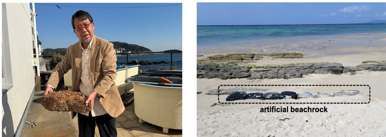
Fig. 26. Coral sand/gravel that solidified within two weeks (left) and artificial beachrock on a shore (right).
