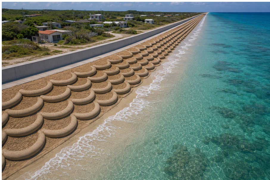
Fig. 21. Conceptual wave-dissipating stepped structure. The step is filled by coral gravel or small sand bags with the outer edge surrounded by sand tubes. Beachrock technology may be applied for both fill and sand tubes to enhance the stability. The permeable structure reduces wave reflection and run-up while promoting sediment accumulation and the formation of a gently sloping shoreline.
