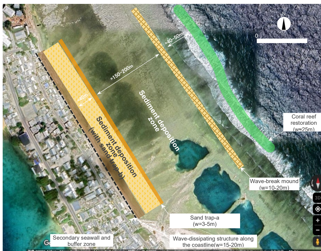
Fig. 29. Conceptual layout of proposed NbS measures for urban coastal areas.
