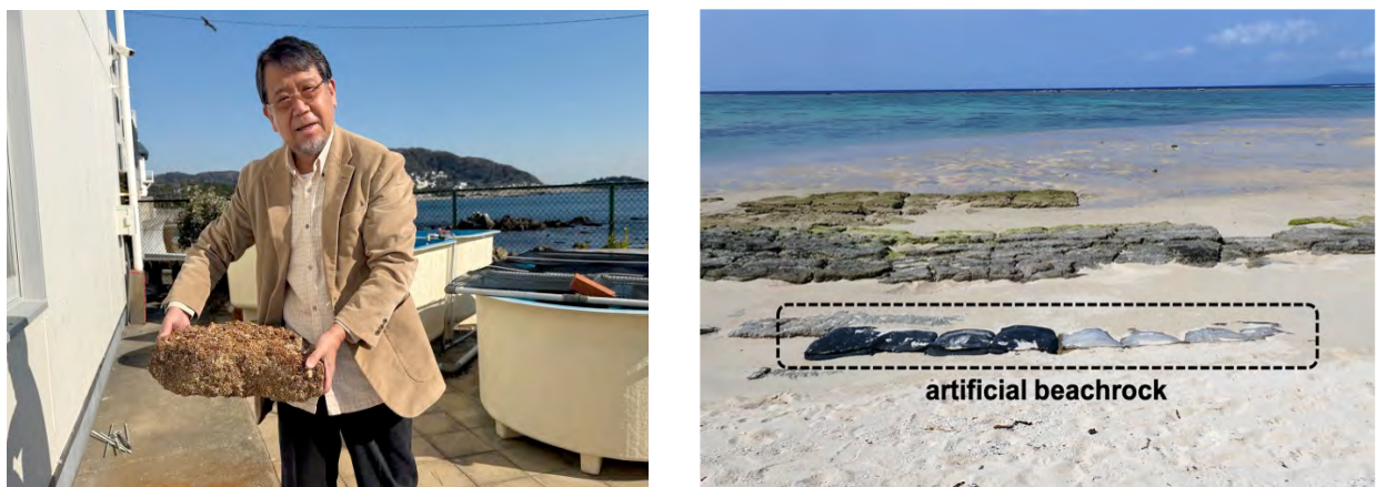
Fig. 21. Coral sand/gravel that solidified within two weeks (left) and artificial beachrock on a shore (right).
