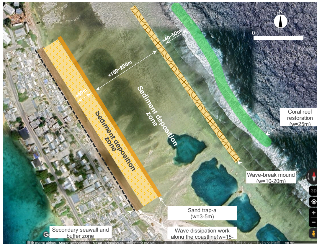
Fig. 24. Conceptual layout of proposed NbS measures for urban coastal areas.
